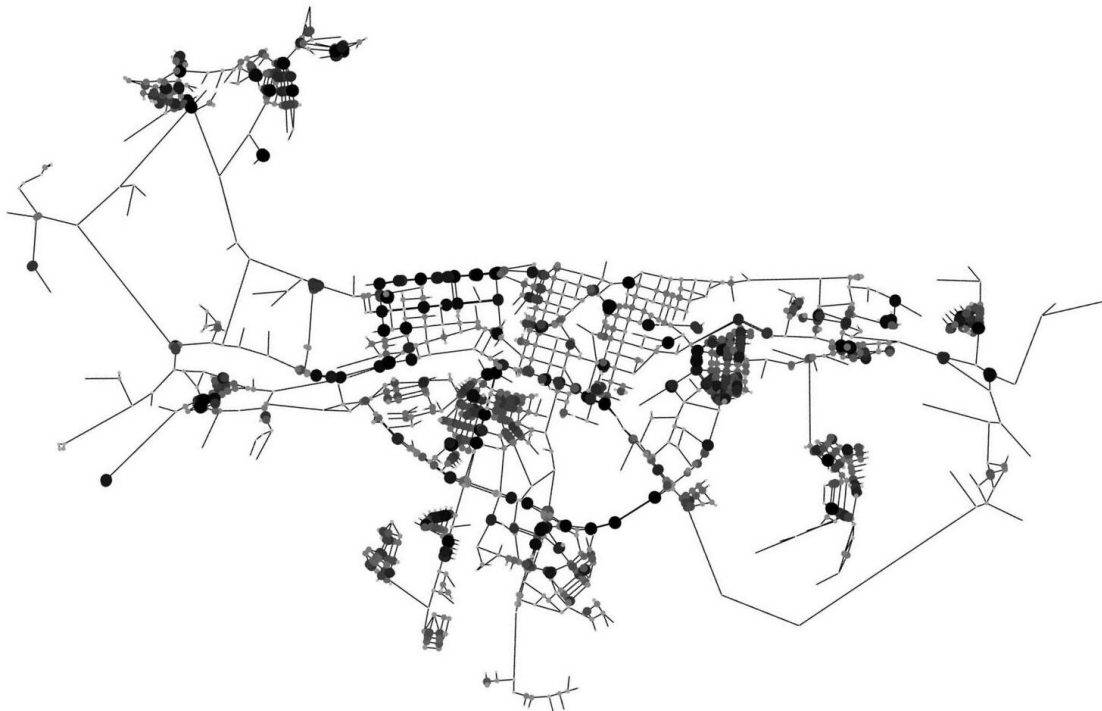
Fig. 9. Heat map of integral centrality values of the Petrozavodsk transport network graph vertices.
