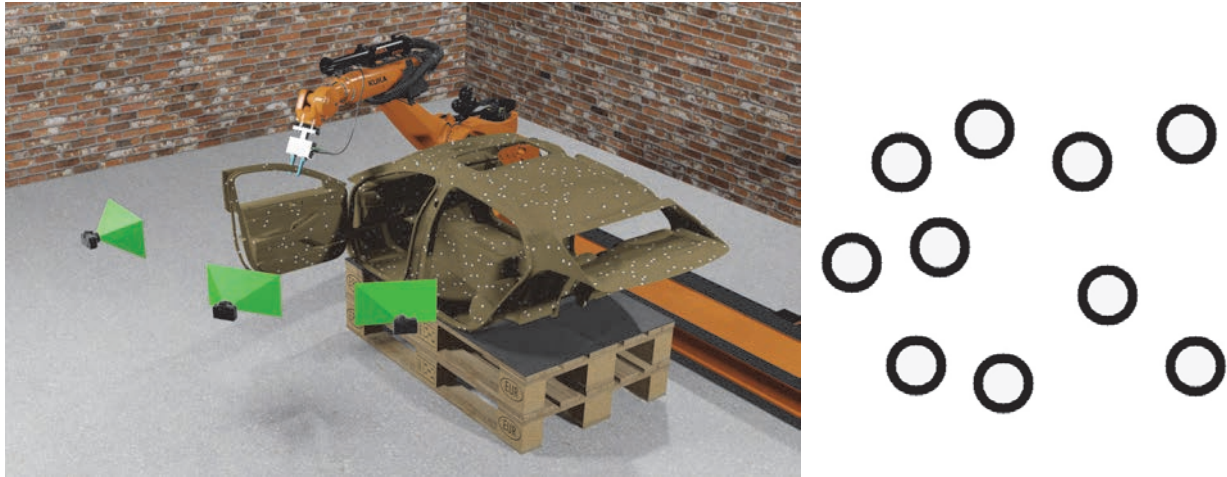
Fig. 2. Left: Example of robot's tool positioning using images from multiple stationary cameras. Right: Circular black-and-white markers (targets) used as features for 3D reconstruction.
