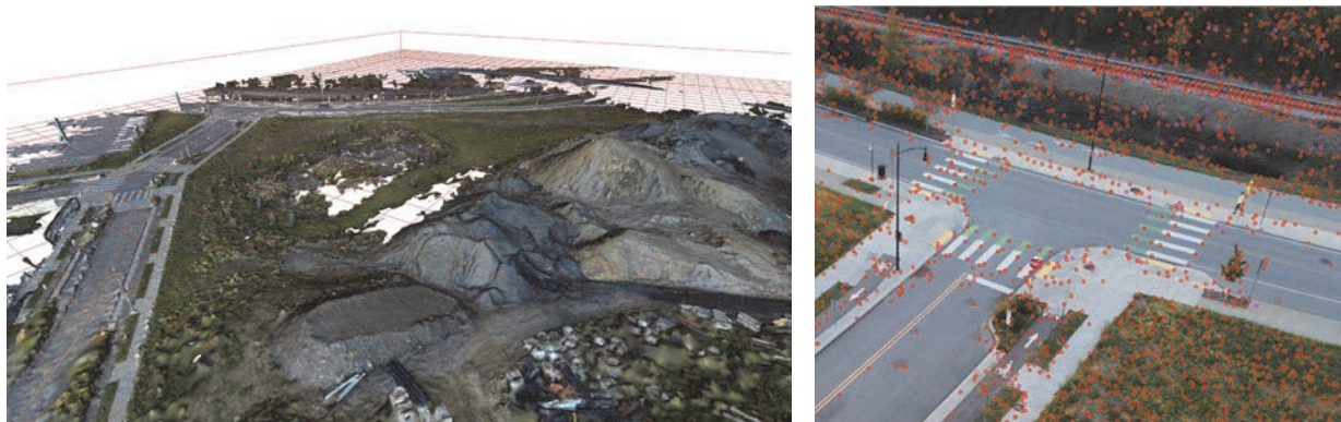
Fig. 1. Left: Polygonal mesh (3D model) of landscape surface obtained through photogrammetry. Right: Original photo (crop) where circles indicate positions of SIFT feature points for matching and triangulation in the photogrammetric optimization problem.
