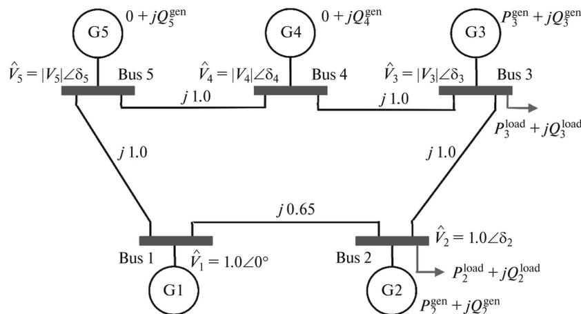
Fig. 4. 5-bus power system test case.
