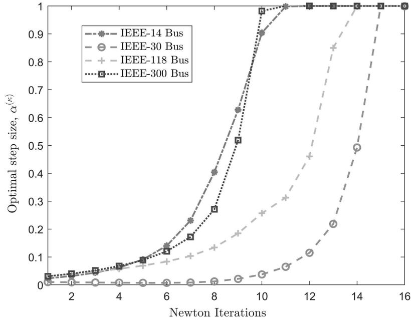
**Fig. 3.** Optimal step size  $\alpha^{(\kappa)}$  selection for each iteration of the TENR method for IEEE test systems.
