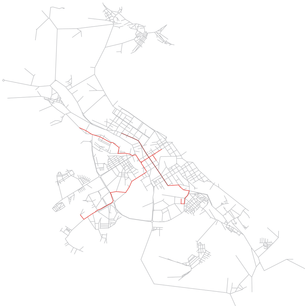
Fig. 9. A subset of the most loaded routes in the transport graph. The route that makes the greatest contribution to the load of the edge with the highest centrality is highlighted in dark red: Pervomaisky Avenue, Antikainen Street and Marshal Meretskov Street.
