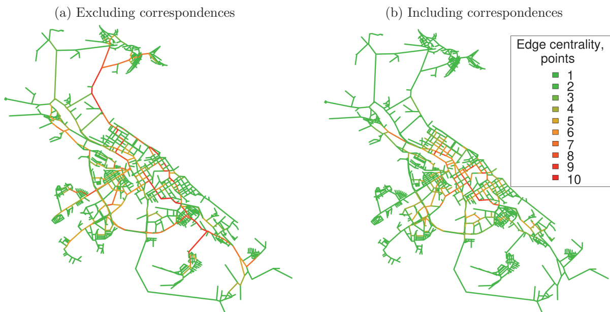
Fig. 2. Edge centralities in the transport graph of Petrozavodsk: 1 point is the minimal centrality, 10 points is the maximal one.
