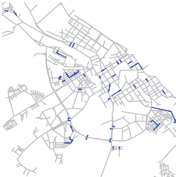
Fig. 7. Reserve road sections: edges that have low centrality in the original graph and change it greatly with random modifications of the graph. These sections may be heavily loaded when other routes are unavailable.
